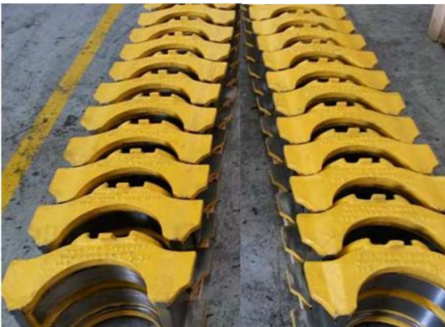
Customised Bearing Adapters: Interface between Short G-Bearings /HH Side Frames
