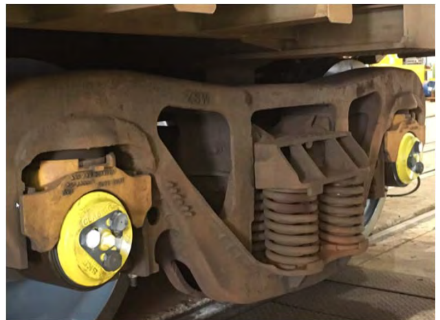
Customised Bearing Adapters: Interface between Short G-Bearings /HH Side Frames
