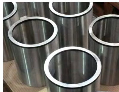
Manufacturing cast adapters and case carburized sleeves
