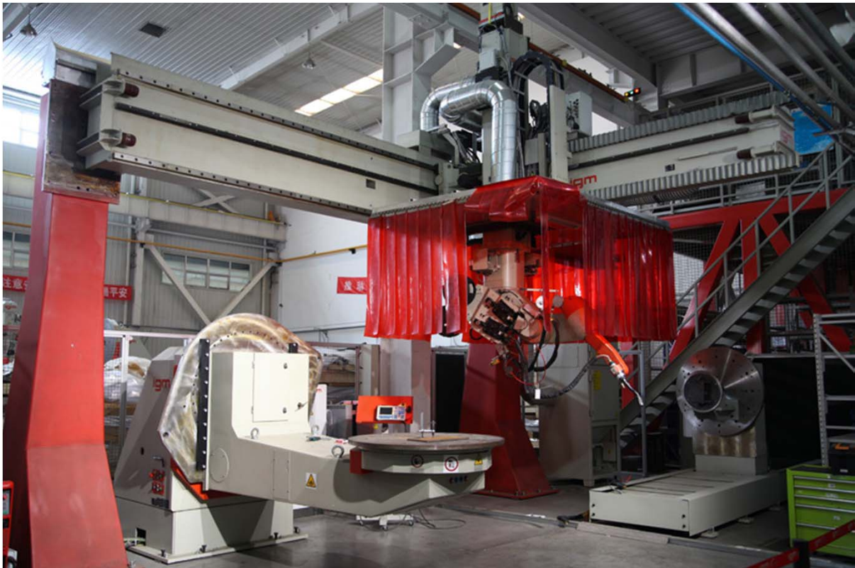
New Bendigo Workshop Layout for Robotic Bogie Manufacturing IGM Machine example below
