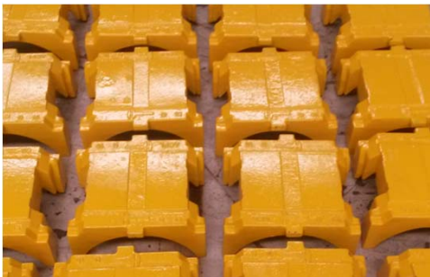
Manufacturing cast adapters and case carburized sleeves
