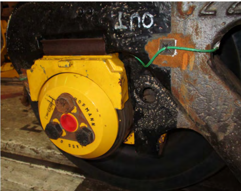
Strain gauge application and on-board stress monitoring during trial
